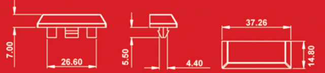
2206 Su Tahliye Plastiği Emptying Hole Cover for PVC Joinary
